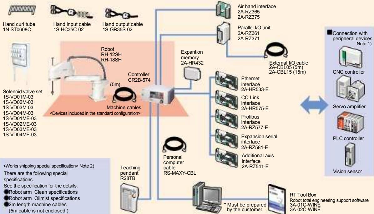
Note 1: Select an appropriate interface according to the I/O on the peripheral device side or network function.
